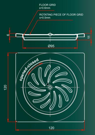
FLOOR GRID, sealing type 150x150/130
